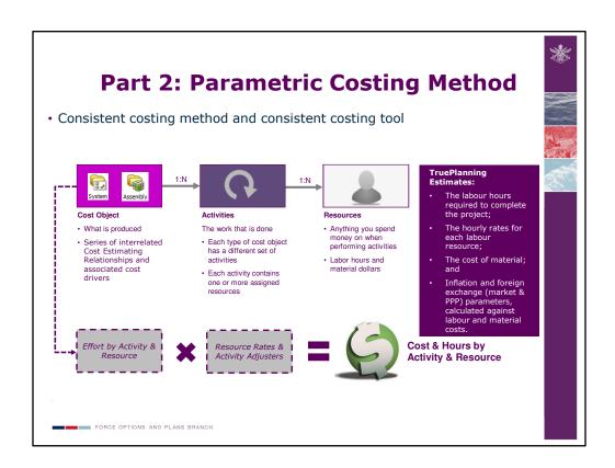
For costing tool, the FSP20 mainly employed a commercially available parametric costing tool, which is TruePlanning. The tool came with a defence capability database which is normalised and updated regularly and usual financial treatments such as inflation rate, forex and purchasing power parity (PPP).
