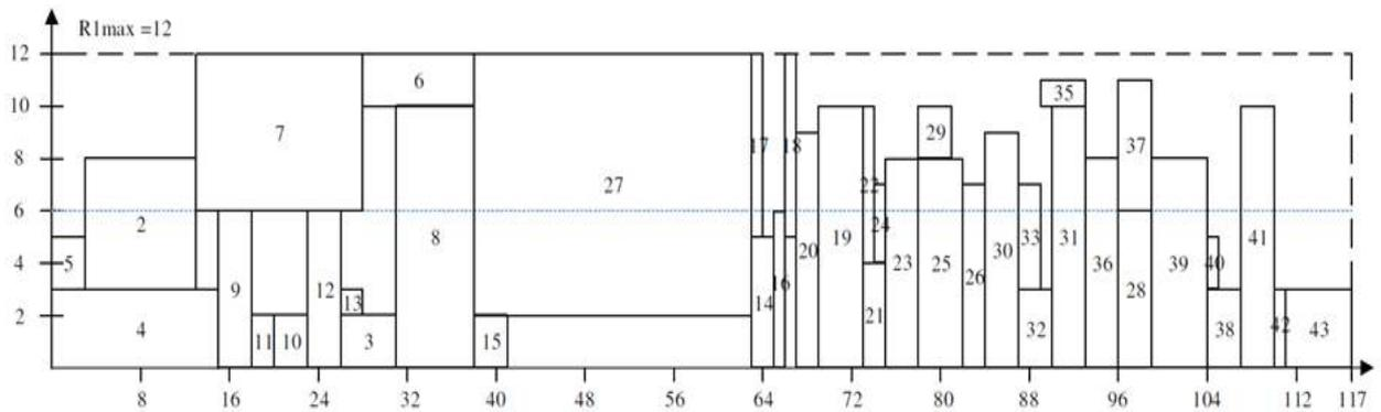
**Fig. 5:** Optimised resource histogram for resource R1 (using a RCPSP method)
