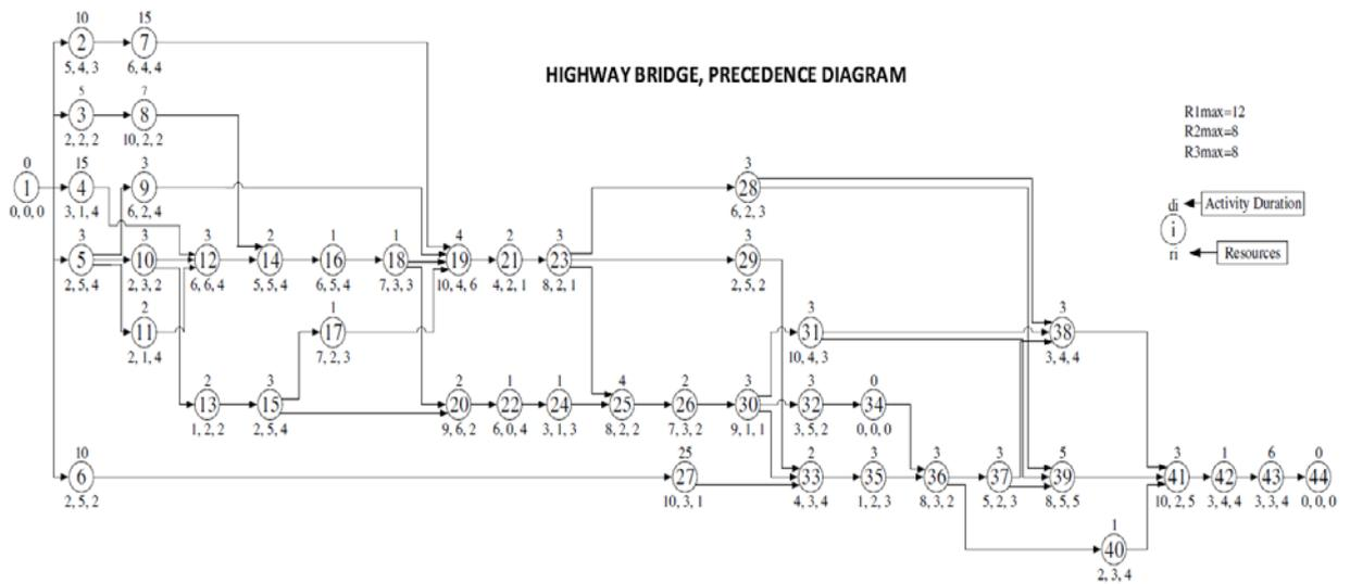
**Fig. 2:** Network diagram of the Highway Bridge project (Tran *et al.*, 2016)
